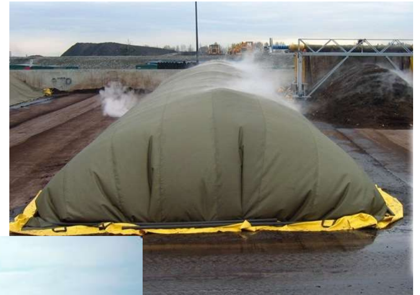
Covered windrow using Gore System (Alberni Clayoquot, Sechelt)
